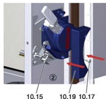
Fig. 184: Install the fusible link holder
