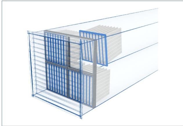
Filter wall type SIF for installation into ventilation systems. Fitting of filter elements for the separation of coarse dust and fine dust and for the adsorption of gaseous odorous substances and contaminants.
