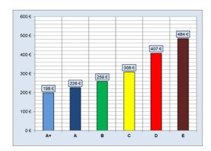
Within a period of one year, one pocket filter of filter class ePM1 75% according to ISO16890, using a volume flow rate of 3.400 m3/h consumes EUR 407 in engery efficiency class D and EUR 198 in engery efficiency class A+. Changing the filters from energy efficiency class D to A+ resukts in an energy costs saving of 51% (EUR 209).
