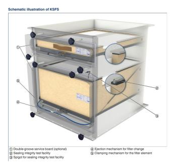
Ducted particulate filters KSFS for critical requirements as filter casings for installation into the ductwork of ventilation systems.
