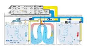
Taking into account the diverse, varying requirements in laboratories, a concept was developed that integrates all important functions in one complete system: the TROX UBox. It can respond to different conditions with real demand-based ventilation and air conditioning, dissipate thermal loads in an energy-efficient manner and take into
