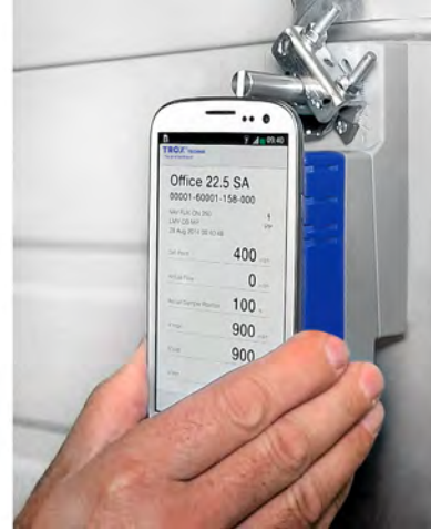
Fig. 21: Connection with NFC-enabled smartphone
