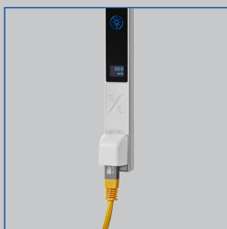
Service socket for controller configuration
